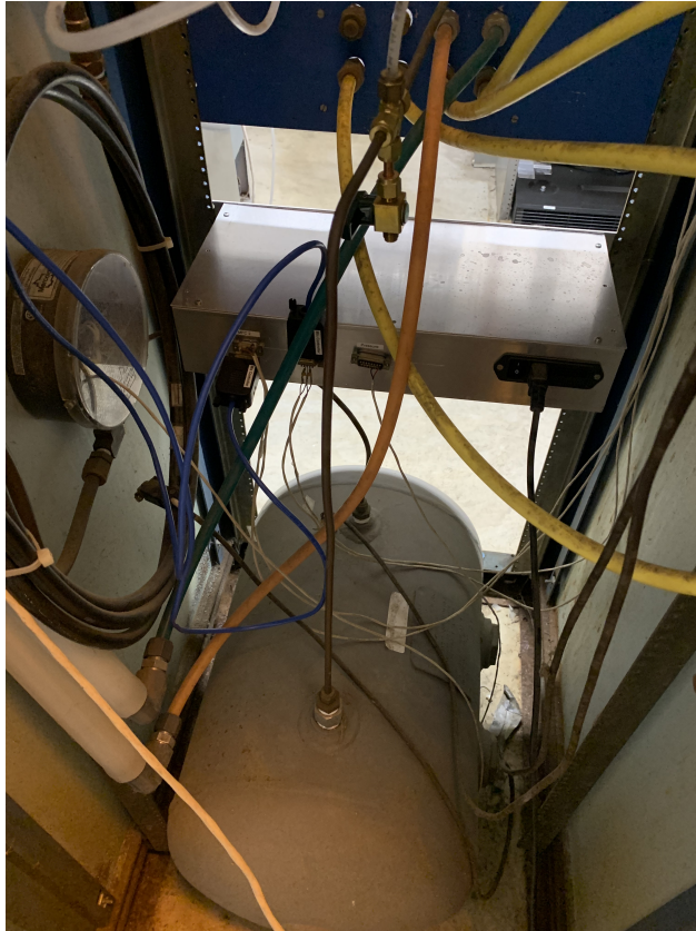
Figure 23: BigBite GEM buffer tank and purge valve.
