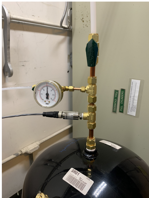
Figure 31: SBS GEM Gas Shut Off Valve, in this picture valve is open
