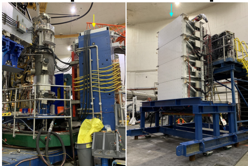
Super BigBite Spectrometer including Super BigBite Magnet and Hadron Calorimeter (HCal)
