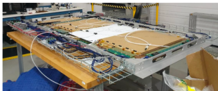
UVA XY-GEM Layer schematic and picture without RF shielding
