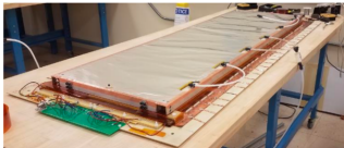
UVA UV-GEM Layer schematic and picture with RF shielding
